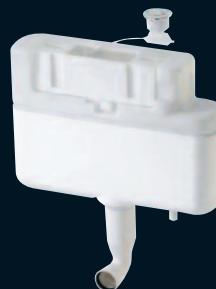
CIS049WH Intra Concealed Cistern £116 • Size 332 (H) x 460 (W) x 127 (D) mm • 10 year Manufacturers Guarantee (excluding rubber parts) • Front or Top Access • Bottom Entry/Feed • Dual Flush - 6/3 Litre • Anti Condensation Jacket • Silent Fill Inlet Valve
